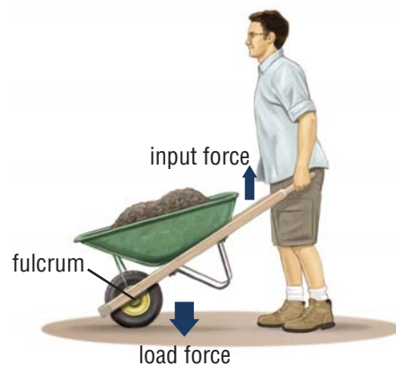
Figure 6 A wheelbarrow is a class 2 lever.
